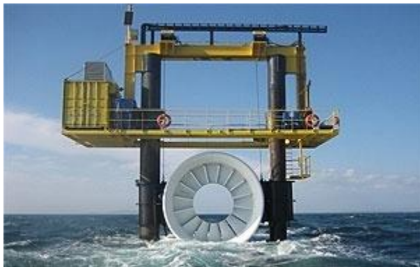
Figure 3: An ocean view of OpenHydro's tidal current turbine installed near the Orkney Islands at the European Marine Energy Consortium (EMEC) test site.
