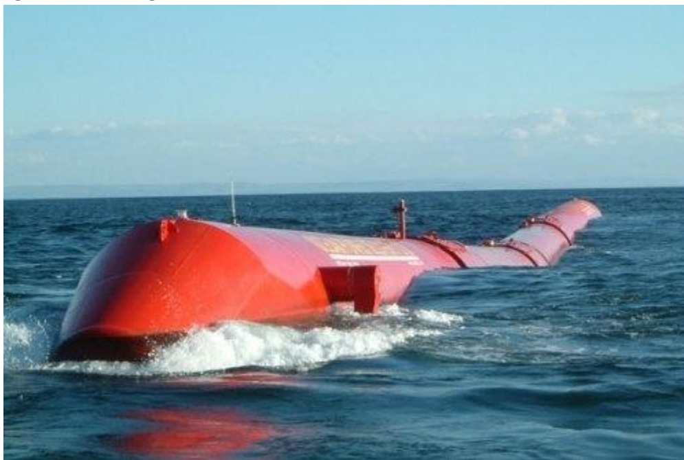
Figure 1: The 750 kilowatt (kW) Pelamis sea “snake” converting wave energy to electricity during sea trials in Aguçadoura, Portugal.
